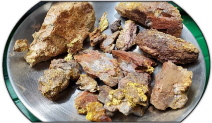
Coarse Gold in Shear Zone Quartz Veins
