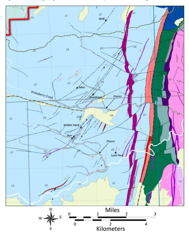
Figure 6-4. Bedrock geological and mine location map of the Lewiston mining district.
