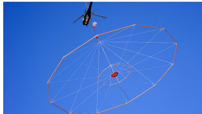
Above: Map of the Seminoe Mountain region. A red ellipse indicates the approximate project area. Below: Example of helicopter-borne TEM survey equipment in flight.
